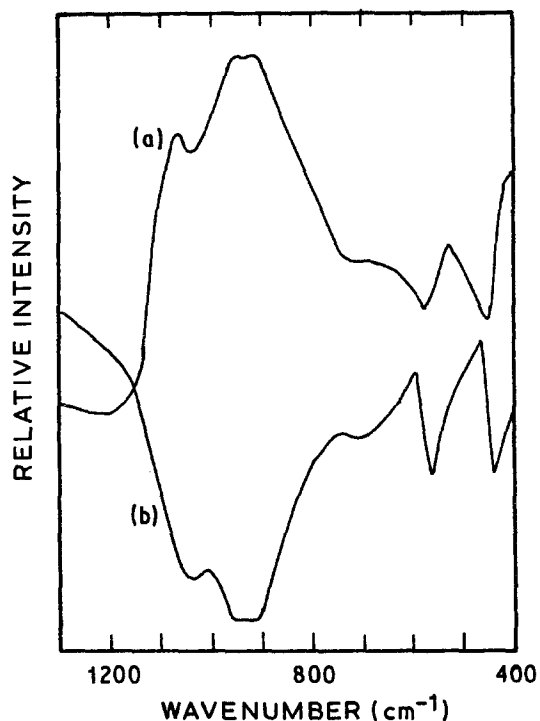
Figure 2 Powder IR transmission and IRRS spectra of sialon with z = 1 in the system \text{Si}_3\text{N}_4\text{-Al}_2\text{O}_3\text{-AlN} .
